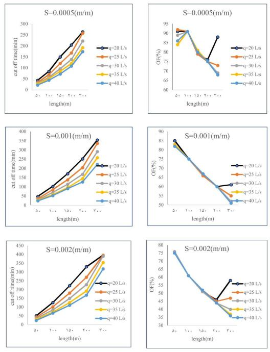
Figure 2. Optimum design and management scenarios with different slopes, lengths, and inflow rates in Field 2.
