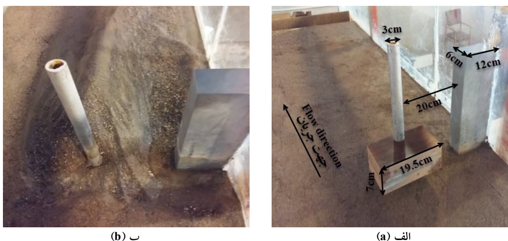
Figure 6. Topography of sedimentary bed a) before and b) after the scour.
